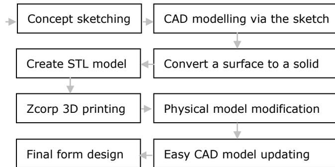
**Figure 2:** The integral form design process with digital fabrication (3D printing)
